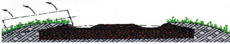
Old condition with high shoulders and deep tracks
